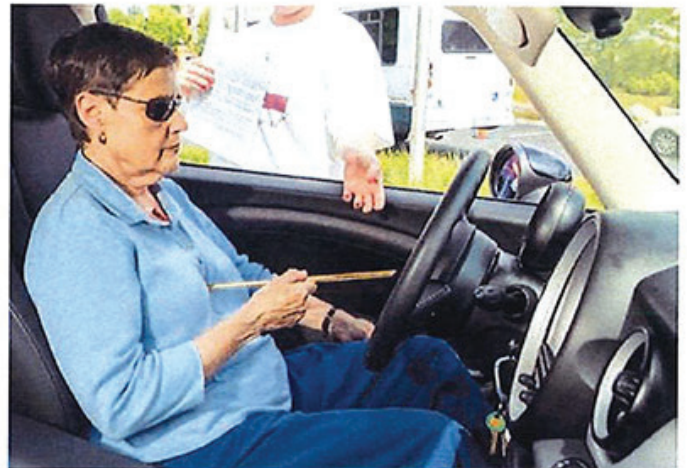
Adequate space between the front air bag/steering wheel and the driver's breastbone; properly adjusted head restraints
